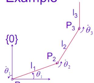
$$v_{i+1} = v_i + \omega_i \times P_{i+1}$$
