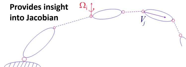
$$\text{Revolute Joint } \Omega_i = Z_i \dot{q}_i$$
